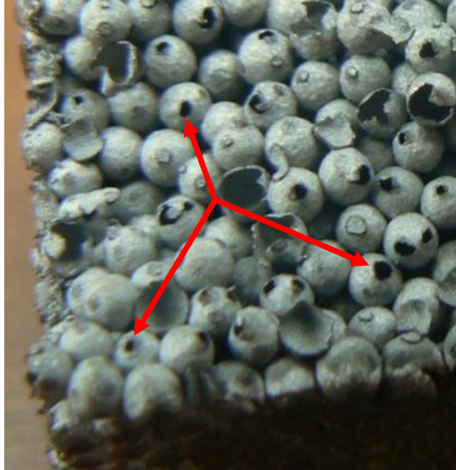
Figure 33: Macro photo of tensile fracture surface. Arrows indicate examples of spheres from which welds have pulled out.
