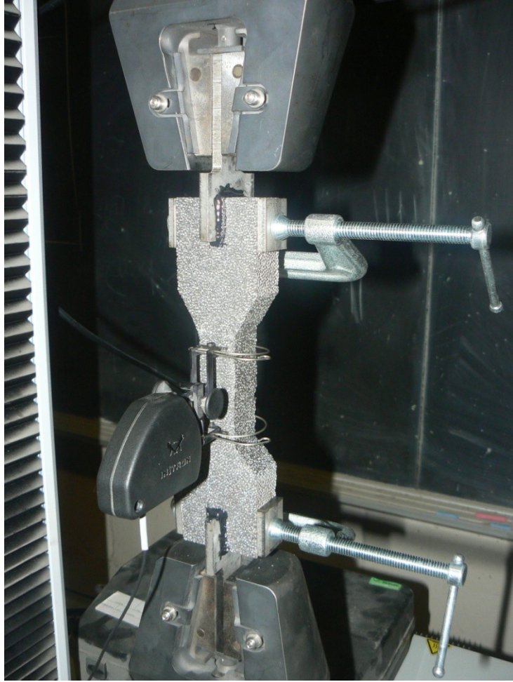
Figure 31: Image of a hollow spheres tension test in progress.
