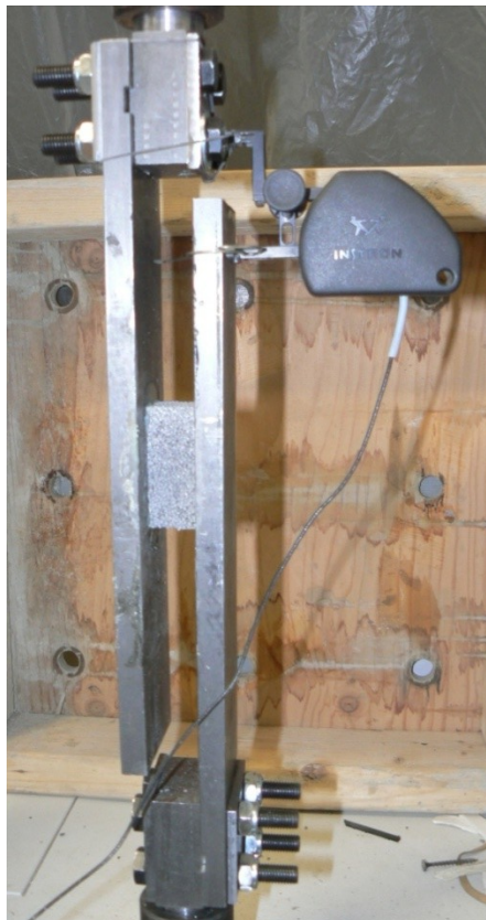
Figure 18: The shear testing apparatus, based upon ISO 1922, loaded with a sample and ready for testing. The extensometer is attached in the upper right.
