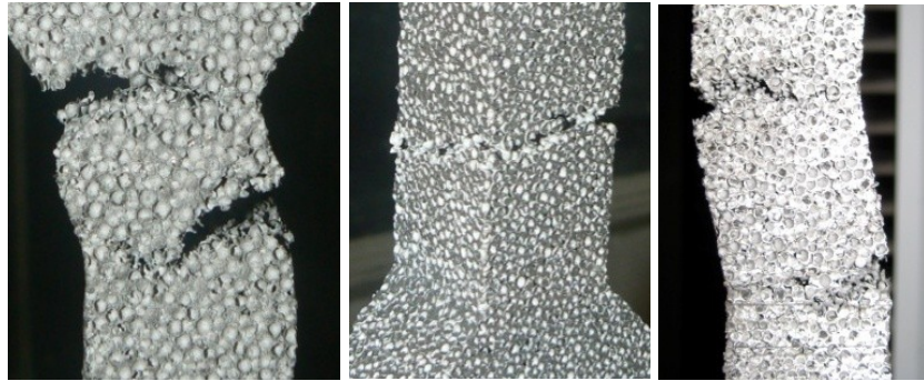
Figure 32: Stress-strain curves for the three tension tests performed (top), with corresponding photos of failed specimens (below, tests #1 through #3 pictured from left to right).
